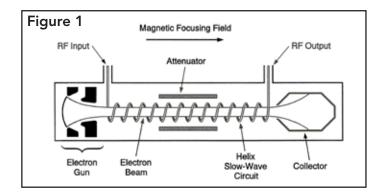
In addition, a magnetic field along the axis of the device (not shown) is used to focus the electron stream. Although TWT's may differ widely in size and construction, depending on the application, the basic theory of operation is the same for all types.
